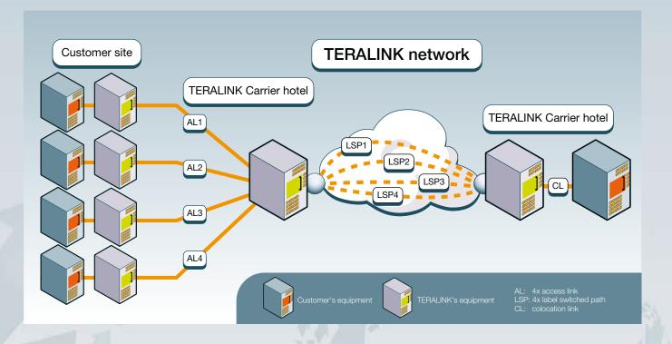
Based on TERALINK's high quality IP/MPLS backbone the TERALINK Virtual Link delivers connections with a capacity ranging from 100 Mbit/s to multiple Gbit/s between numerous cities throughout Europe. It consists of protocol transparent point-to-point and multipoint Ethernet connectivity with dedicated virtual channels for each customer.
